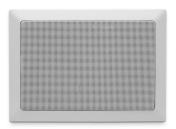
CMR20T is a very compact and performant two-way rectangular 100 volt built-in speaker, provided with a 5.25" paper cone woofer and 1" tweeter. The two-way aspect makes the loudspeaker very suitable for the reproduction of both background music and microphone calls.
